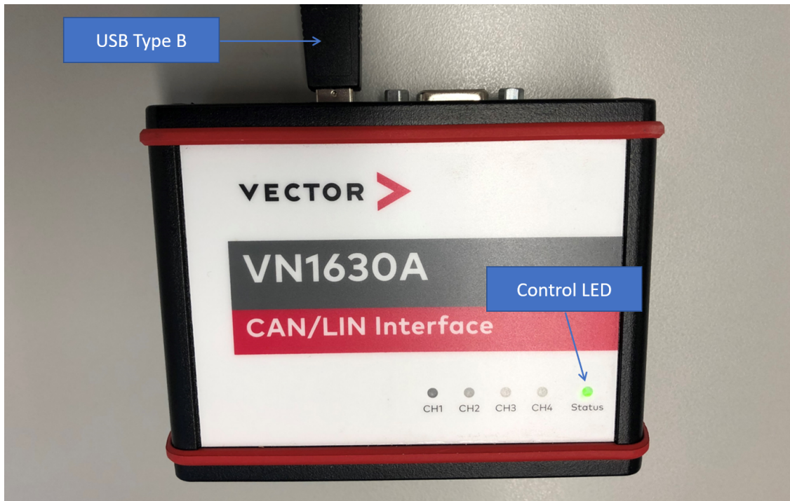
Figure 2: VN1630A Connection to Host Computer. (VN1640A similar.)
