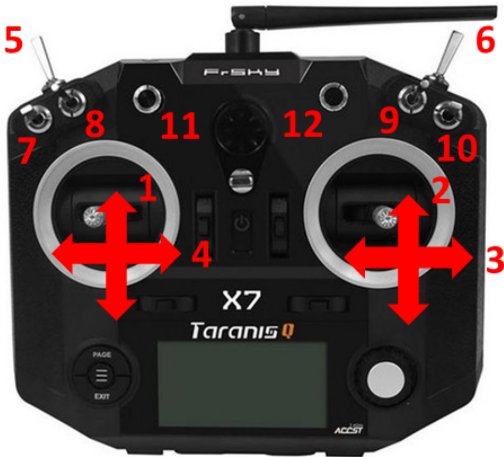
Figure 8: Channel Layout of Exemplary Remote Control (Model: Taranis FrSky Q X7).
