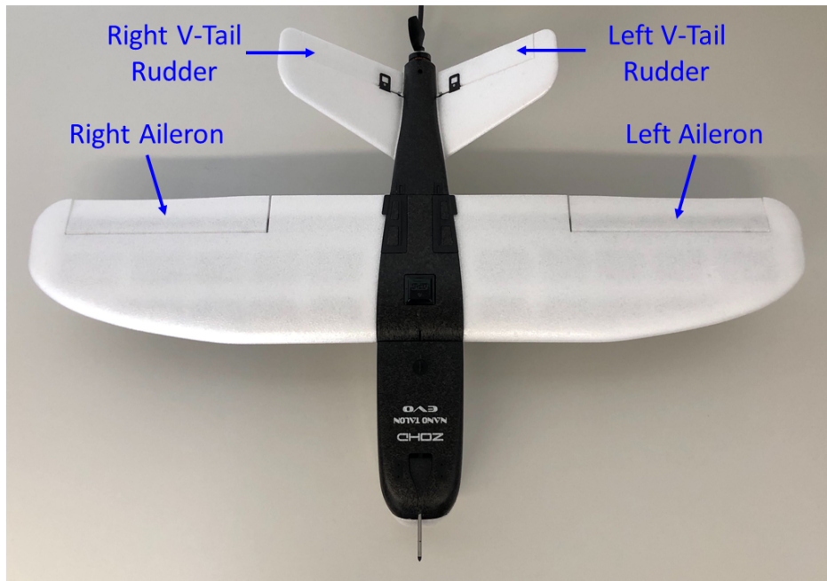
Figure 7: Assignment of the Rudders.
