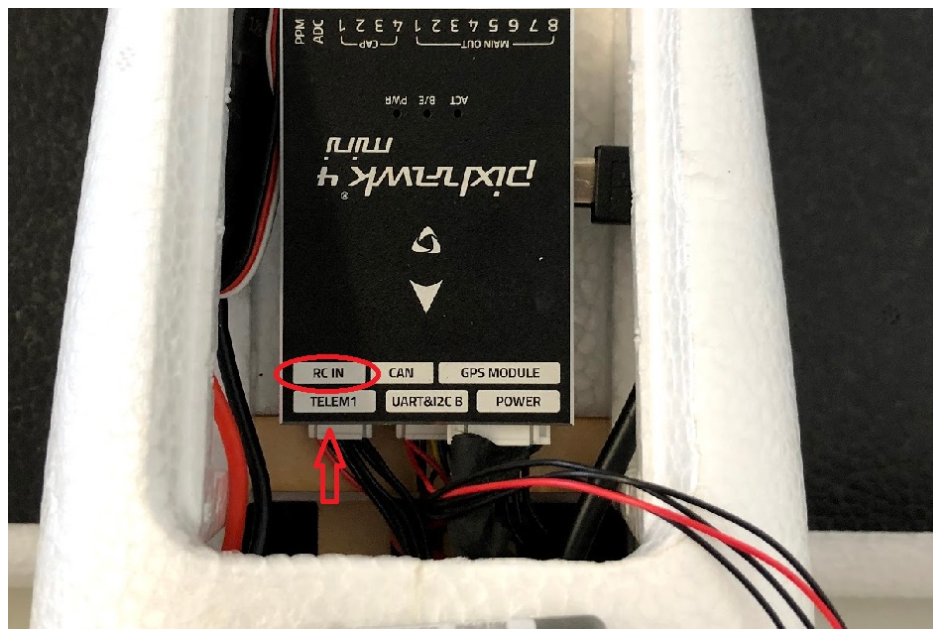
Figure 6: Connection of the RC Receiver to Pixhawk 4 Mini.
