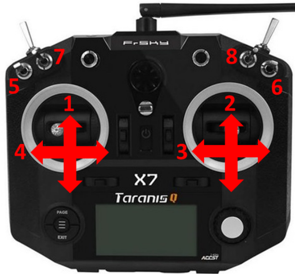
Figure 5: Channel Layout of Exemplary Remote Control (Model: Taranis FrSky Q X7).
